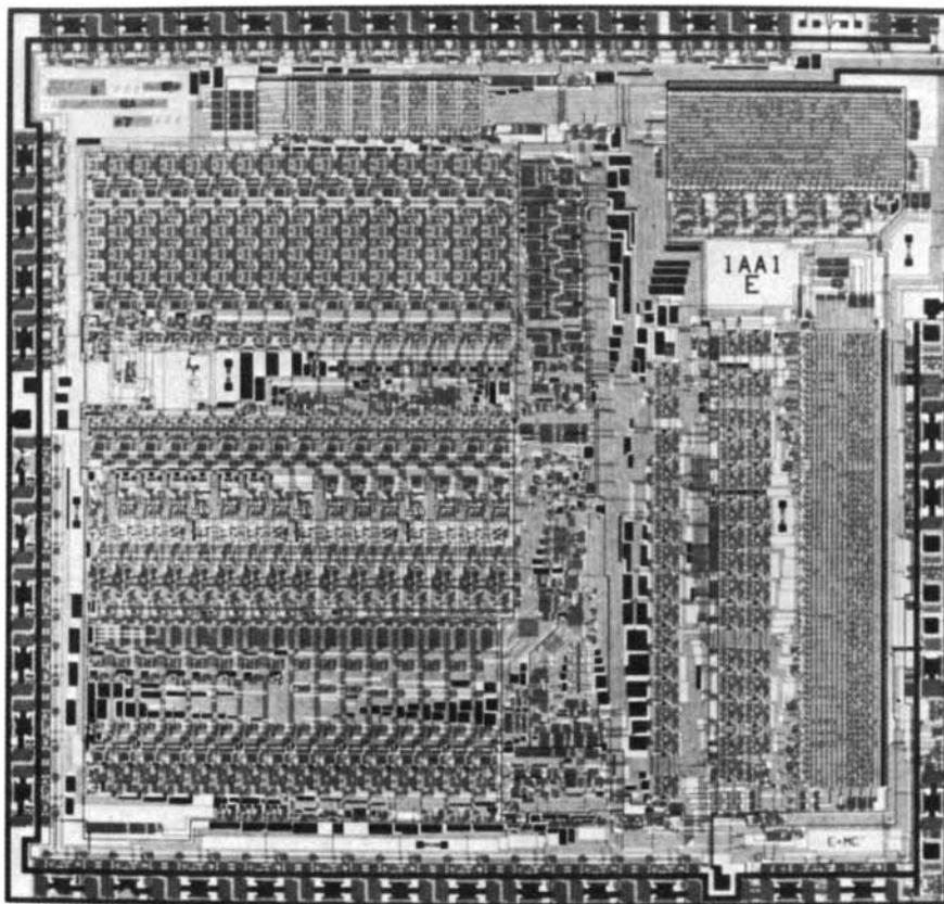
Actual size of the MC<sup>2</sup> chip is
