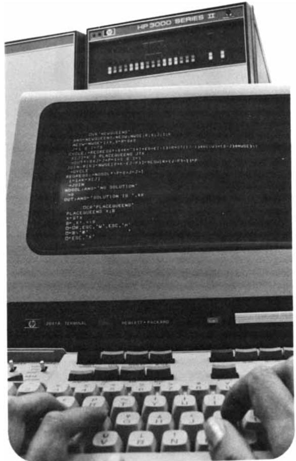
standard ASCII character sets. Additional special function keys can be programmed to speed data entry and reduce opportunities for error. Optional minicartridge tape transports provide storage that allows the user to prepare data off-line, transmit it rapidly to the computer in batch, and keep or transfer development programs on the pocket-sized cartridges.
