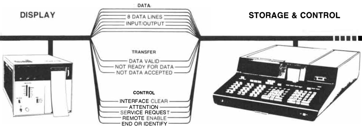
matic system may include as many as 15 instruments possessing stimulus, measurement, display, storage, and control capabilities. Whether a calculator, computer, or the processor of a "smart" instrument, the controller operates the entire system through an interface connection (a single I/O card)—an obvious economy compared to non-bus systems that require one I/O card for each instrument.
