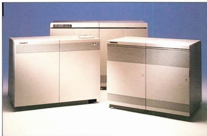
The HP 3000 Series 70 (background), shown with the new Series 930 and 950 computers, is a powerful system for large business applications.
