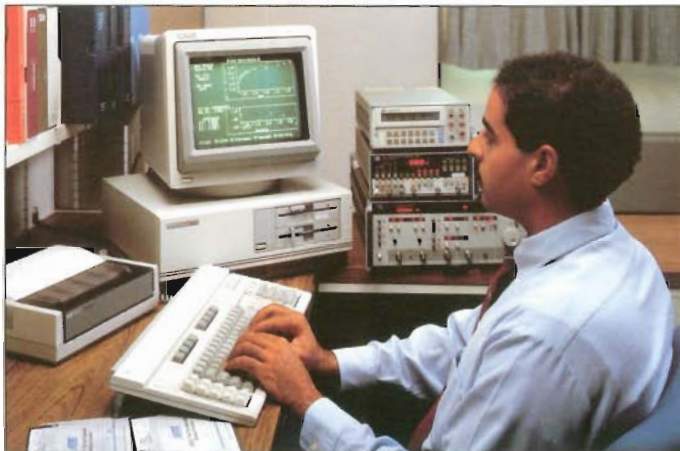
An engineer uses ASYST to collect data from a waveform recorder and analyzes the results on the HP Vectra PC.
