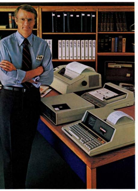
The Personal Computer For Professionals: HP-85 specifications: Memory –16K RAM expands to 32K, 32K ROM expands to 80K; CRT –32 chars./line, 16 lines; graphics –256 X 192 dots; thermal printer –2 lines/sec.; magnetic cartridge capacity –200K; 1/O –HP-IB (IEEE 488), RS-232, 16-bit GP-IO, BCD; Application Pacs include Statistics & Regression Analysis, Finance, Math, Linear Programming, Text Editing, Waveform Analysis, Circuit Analysis, BASIC Training, & Games.
