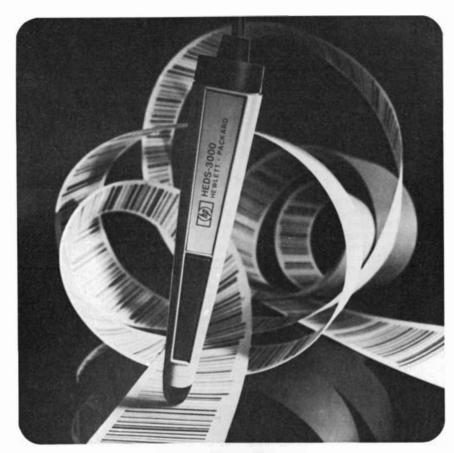
wand will soon be available as an input device for the HP-41C fully programmable hand-held calculator.)
