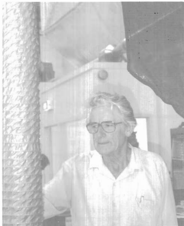
• Bill Allison alongside delivery tube; large elevated holding hopper means packing doesn't have to stop for shells to be reloaded.
