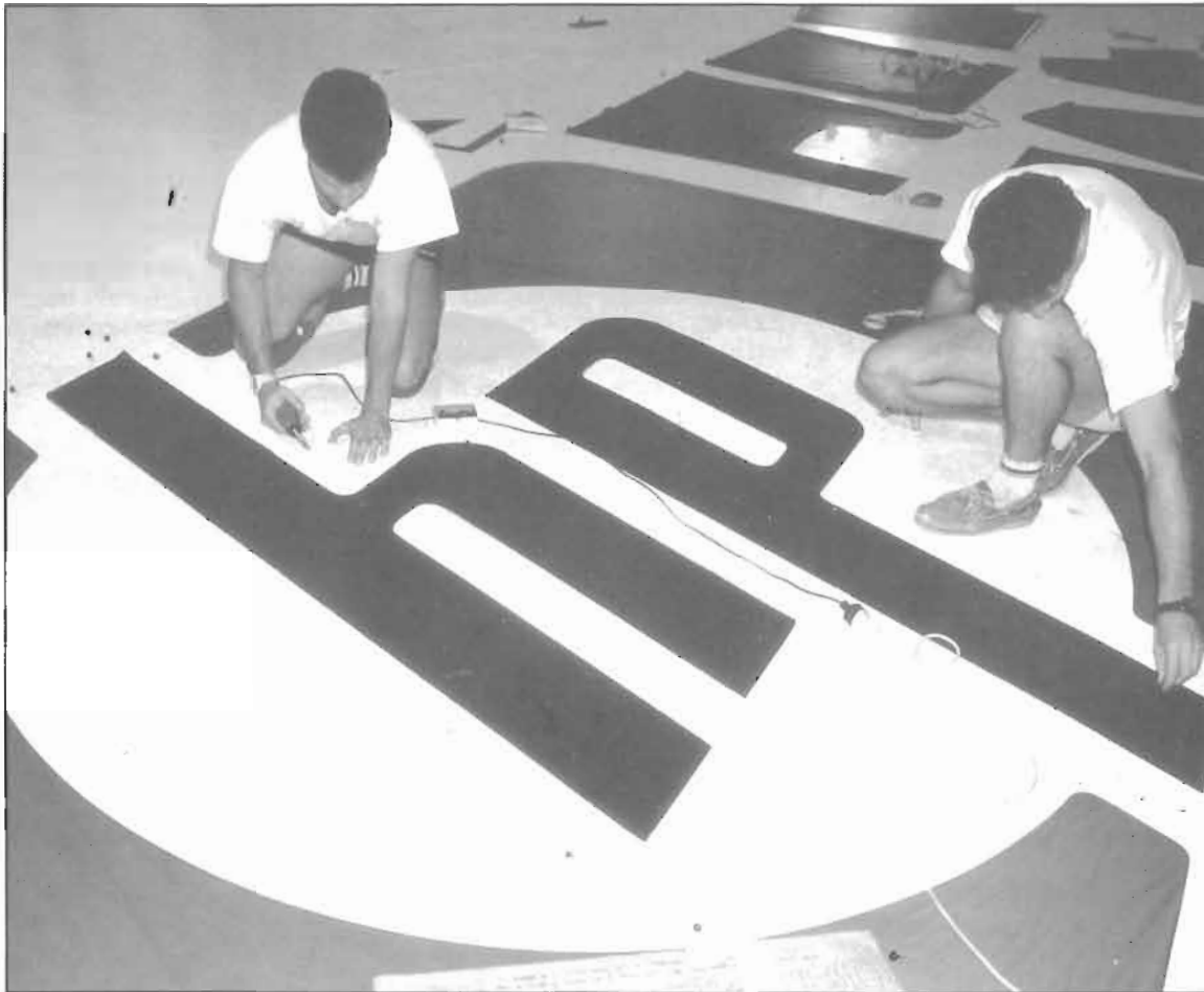
Sailmakers stitch the HP logo to New Zealand's giant genoa, which is big enough to enclose a 40-sq house.
