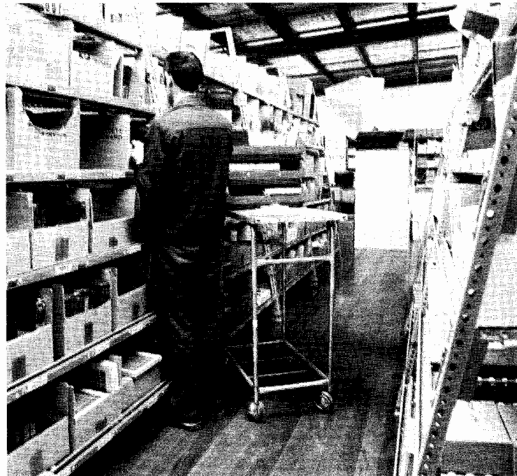
● The system provides 192 picking positions in the carton live storage section.
