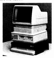
The Display Tilt Unit and the Display Swivel Unit (92171V and 92171W) allow you to tilt the HP 120 CRT display up 10 degrees or down 10 degrees from a horizontal position as well as turn it 360 degrees (cabling may limit full rotation). This allows adjustment for glare and reflection and helps in reducing back and neck fatigue—without increasing the system footprint.
