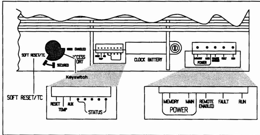
Figure 4-3. Front Panel Layout
