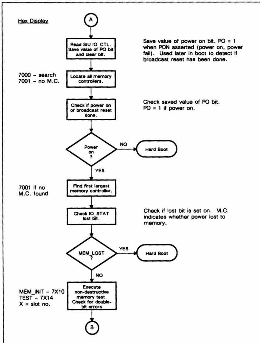
Figure 4-12. Selftest Detailed Flowchart (cont'd)
