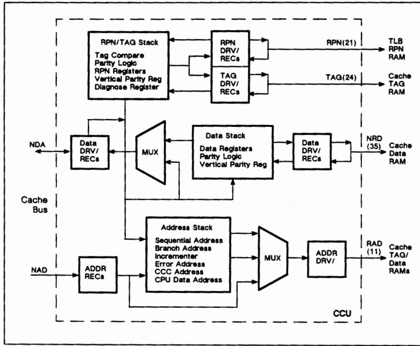
Figure 9-6. 825/925 CCU Chip Simplified Block Diagram
